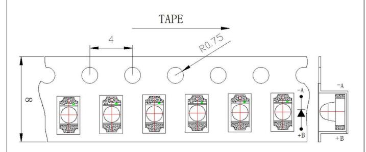
□ □ □ □ □ □ Tolerance unless mentioned is ±0.1mm; Unit = mm
